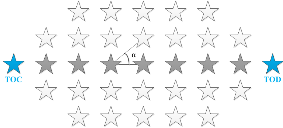
Fig 5 Search space for the lateral reference trajectory created around a geodesic reference trajectory
