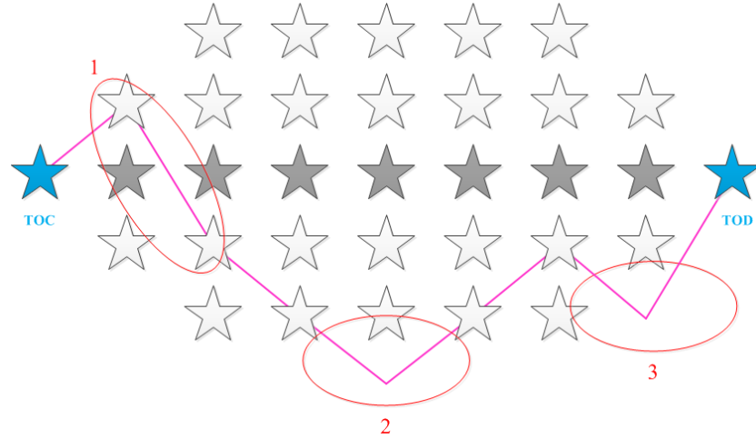
Fig. 13 Lateral Reference Trajectory With Waypoint Selection Discrepancies
