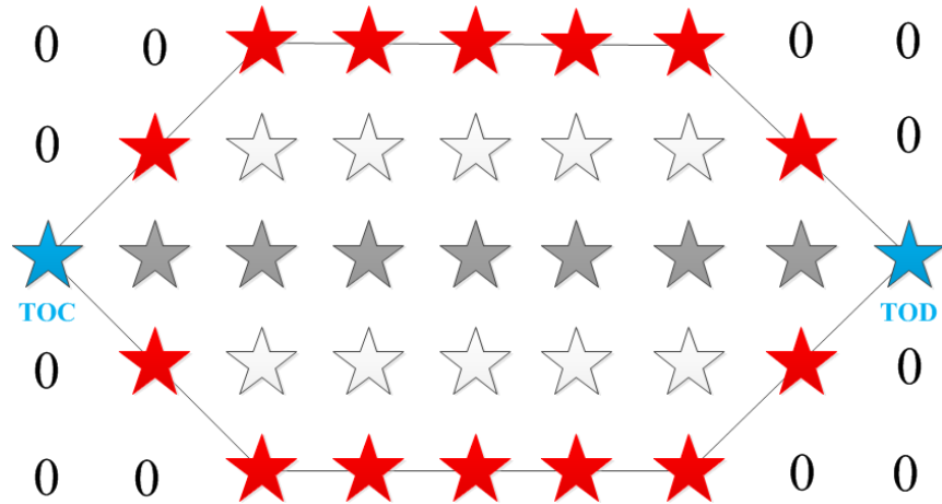
Fig. 6 Search space for the lateral navigation with the boundaries
